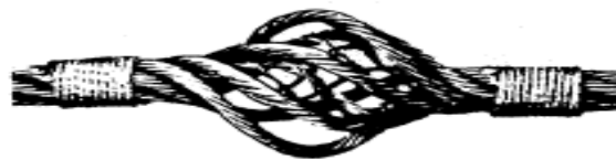
A birdcage caused by sudden release of tension and resulting rebound of rope from overloaded condition. These strands and wires will not return to their original positions.
