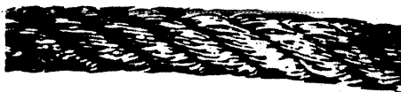
Rope subjected to drum crushing. Note the distortion of the individual wires and displacement from their original position. This is usually caused by the rope scrubbing on itself.
