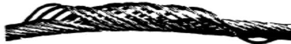
Multi-strand rope "birdcages" because of torsional unbalance. Typical of buildup seen at anchorage end of multi-fall crane application.
