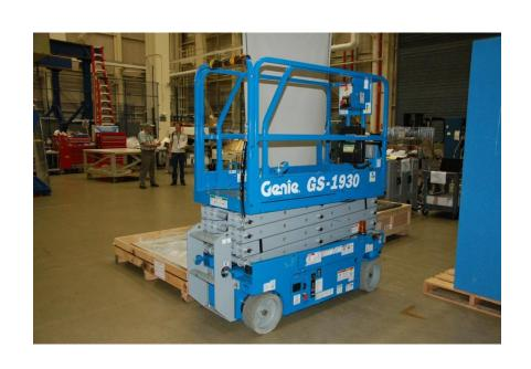
MAP's include: scissors lifts, bucket lifts (JLG, etc) and other powered devices used to position personnel at elevated work locations.
