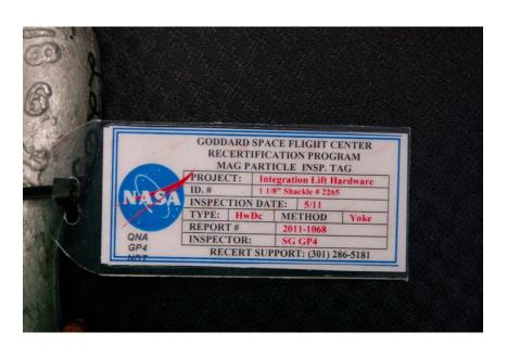
NDT Inspection tags are provided for all critical lifting components
