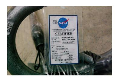
Lift Slings tested as a complete assembly will be tagged with a single RECERT Proof Tag.
