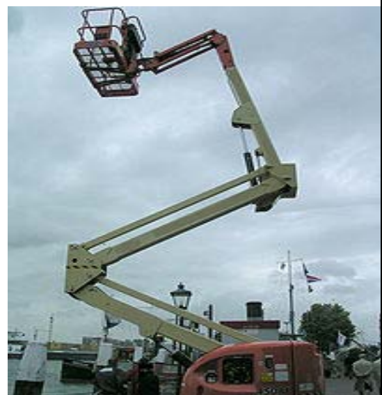
Articulated lift being demonstrated
